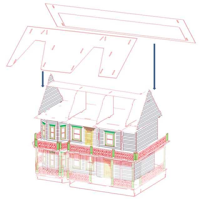
Install front and rear roof panels.
