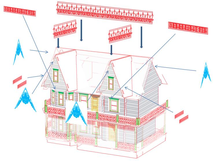
Install roof running rails and front facing fretwork.
