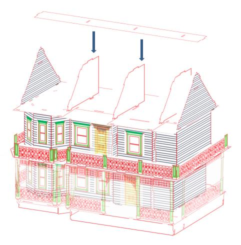
Install 3<sup>rd</sup> floor roof. Note that the top back goes facing up and to the rear for proper alignment.
